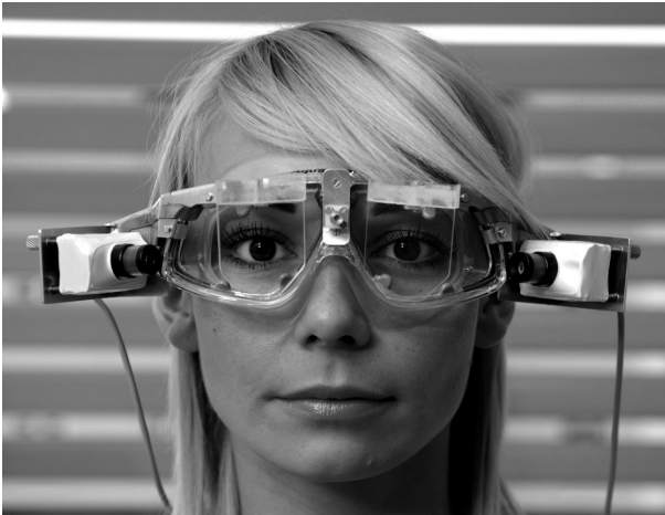
Figure 1: Image of the EyeSeeCam - VOG system which is available at our institution.
